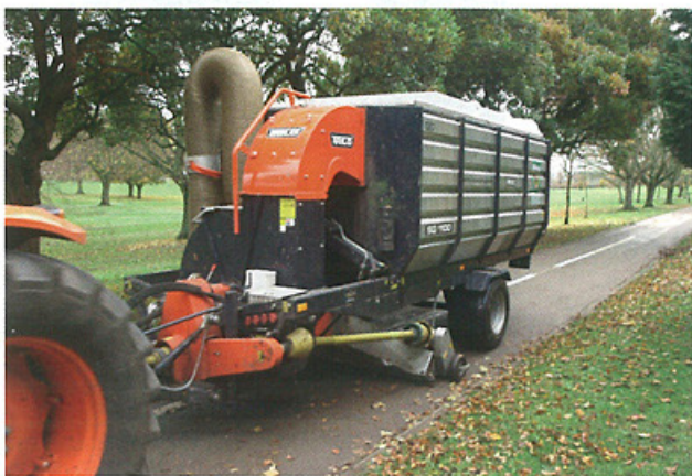
Suction hose parked up, the vacuum sweeper-collector gathers leaves from hard surfaces through its 2m wide suction head.
