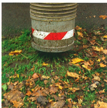
Tremendous suction is produced at the nozzle of the 200mm diameter hose to gather up wet or dry leaves and other debris.
