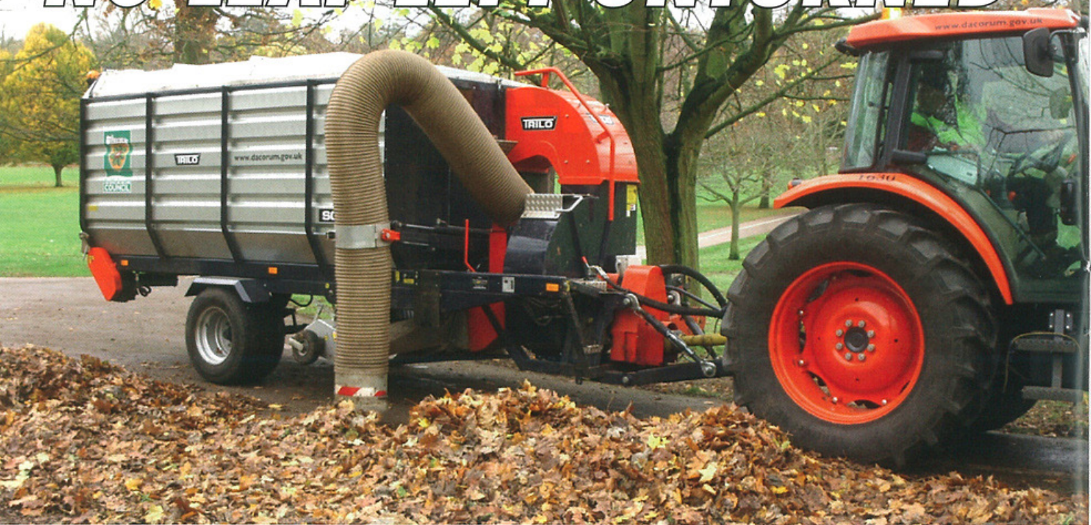
The action and movement of the hydraulically-operated suction hose arm on Dacorum Borough Council's Trilo SG1100 vacuum sweeper-collector is controlled from the tractor's cab.
